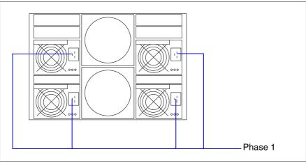
Figure 70: Basic unit with a single phase input
